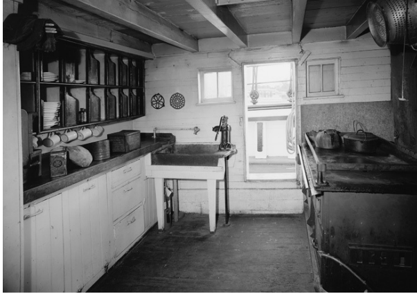
Figure 4.6. Schooner Thayer's galley with special shelves for plate storage. This lumber and fishing schooner features an alternate design of the shelves for the dishes on which cabin meals were served. Call Number: HAER CAL,38-SANFRA,199—19 in Collection: Historic American Buildings Survey/Historic American Engineering Record/Historic American Landscapes Survey . Library of Congress Digital Collections. http://www.loc.gov/pictures/item/ca1506.photos.041956p/ .
